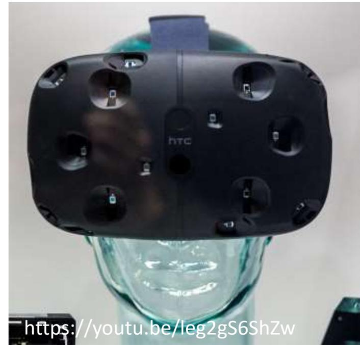
We perceive 3D if an image on a display changes synchronously with our head motion. Therefore, VR should come with head-tracking:
